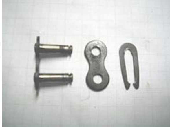
Fig. 52: The removable master link is shown on the right.
