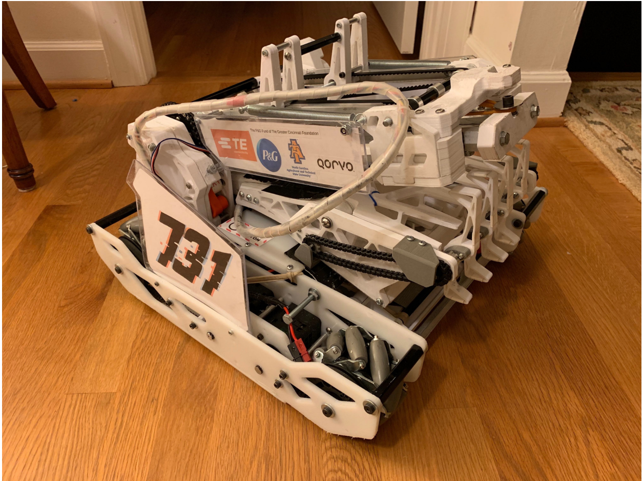
Fig. 16: 731 Wannabee Strange, Rover Ruckus, Design Award Finalist (Houston) 3D printed (PETG and TPU) and machined (milled) arm/intake Custom HDPE drive train (CNC routed)
