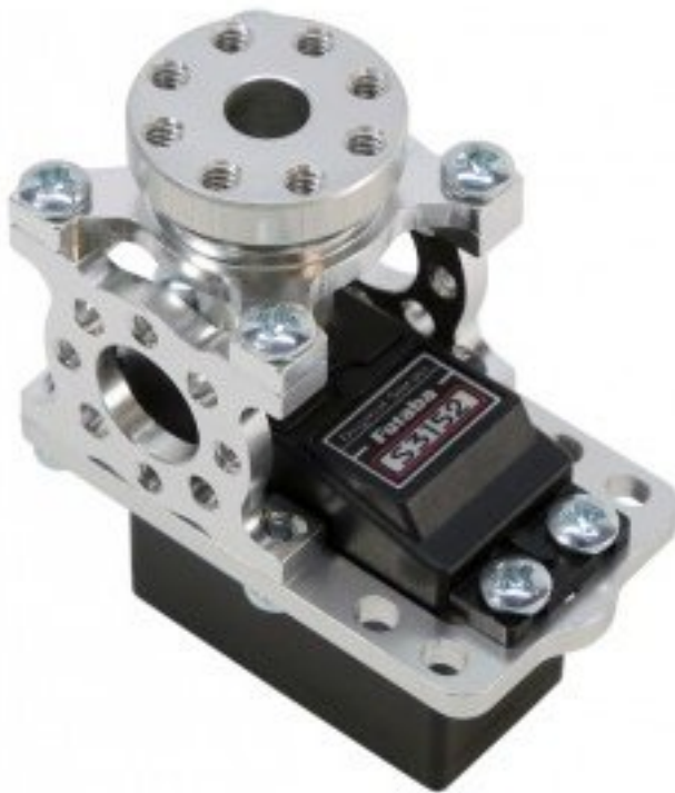
Fig. 20: A servo in a ServoBlock
